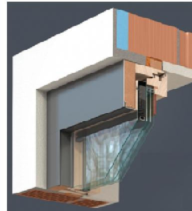
1. New window is installed in the same position as the old window.
