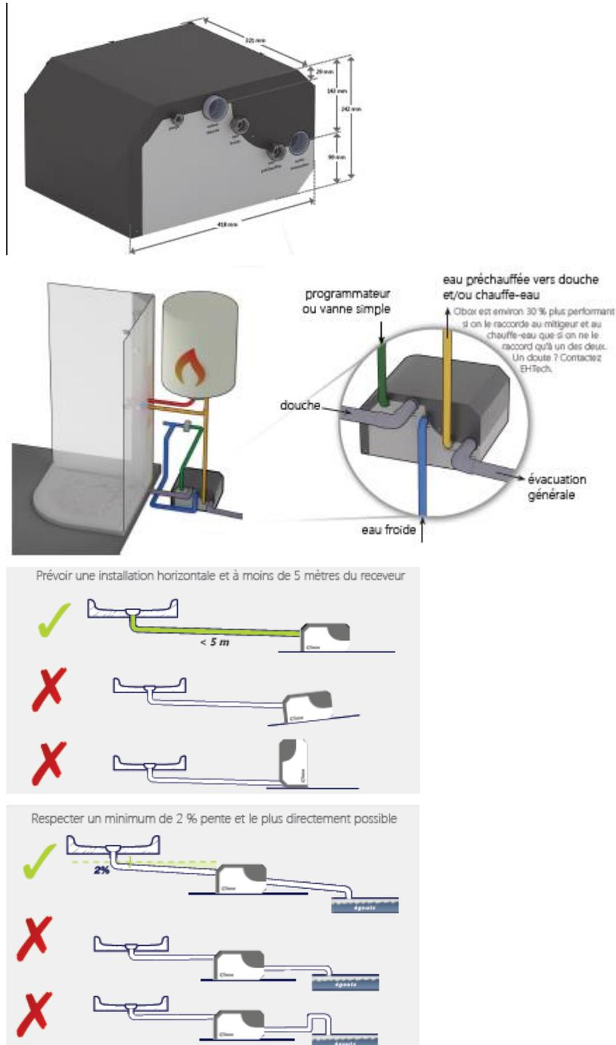
Figure 28 : View of the exchanger unit, recommendations for installation. Source : EH Tech
