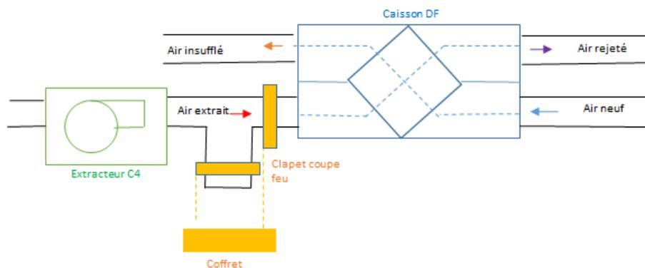
**Figure 23 : Usual situation with a MVHR that is not fire-resistant. Additional exhaust ventilator is required, plus fire dampers. Source : France Air**
