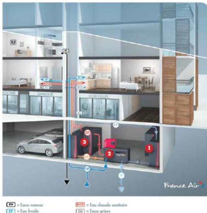
Figure 27 : Integration of Sourcéo in a multifamily house. Source : France Air
