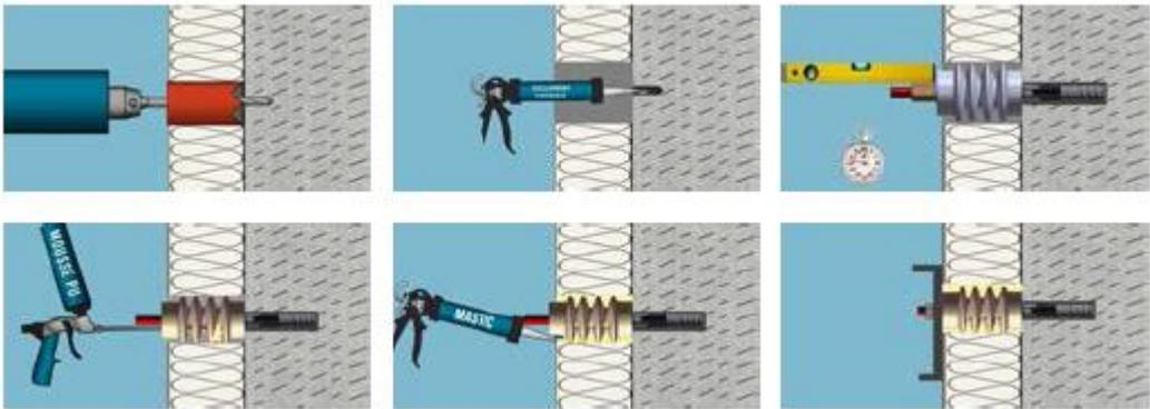
Figure 17 : Installation instructions. Source : IT-Fixing
