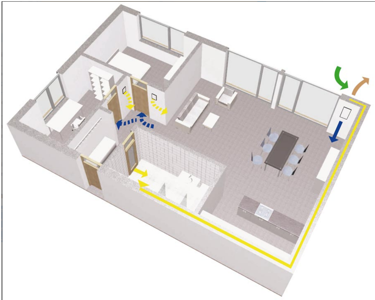
Figure 13: freeAir100 and freeAir plus layout
