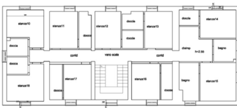
Figure 9: Second floor plan, existing building.
