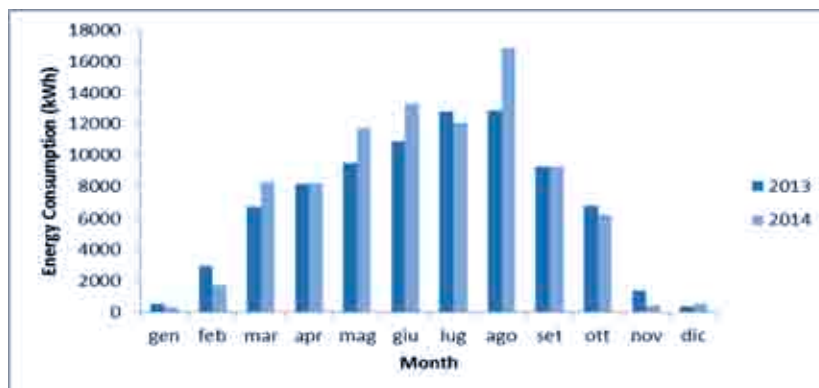
Figure 37: Monthly electricity consumptions of the existing building for 2013 (blue) and 2014 (light blue).
