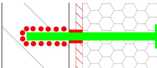
**Figure 10: specialised self-sealing dowel**
