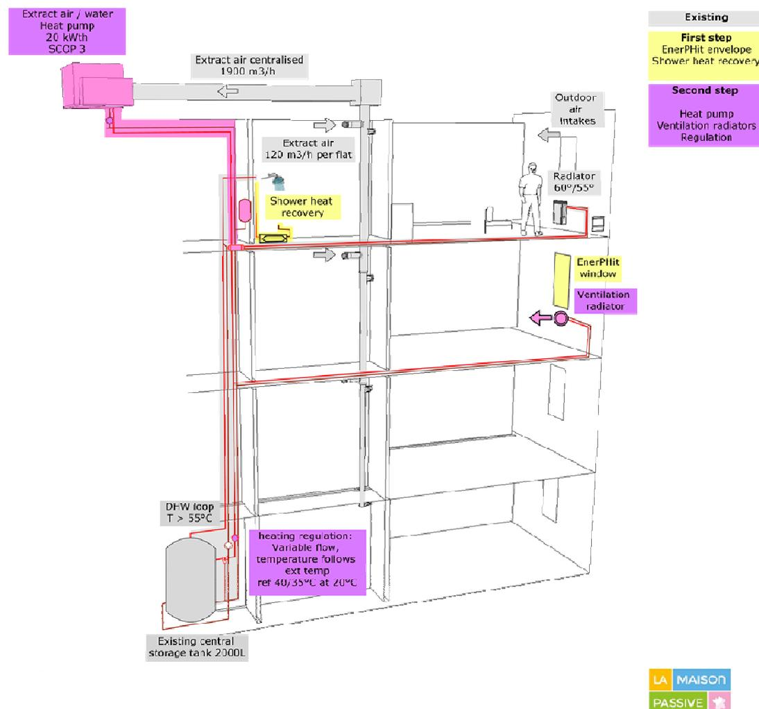
Figure 4: Connection of heat pump to existing circulation hot water loop
