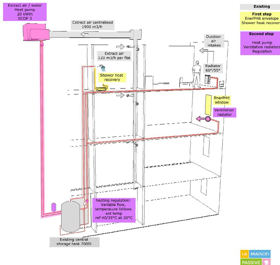
Figure 1: System integration in a 4 storey apartment building, step by step retrofit
