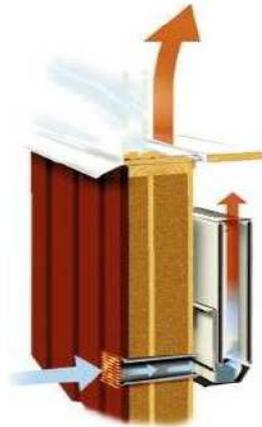
Figure 2: Schematic diagram of a ventilation radiator
