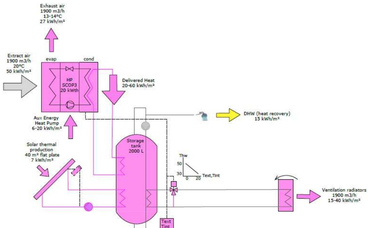
**Figure 3: Energy diagram of solution integrating solar thermal panels**
