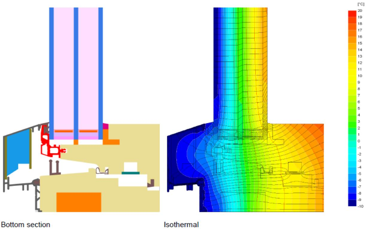
Figure 18 Thermal simulation of the Smartwin window
