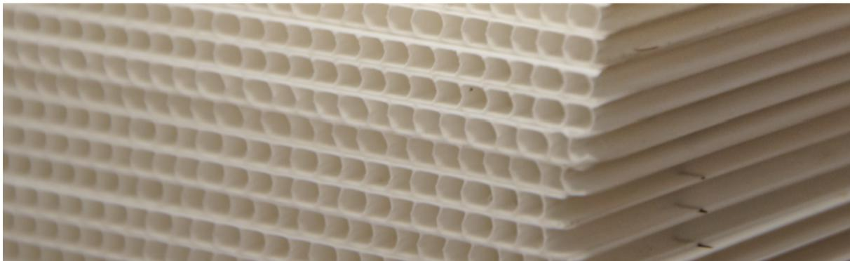
**Figure 1: Polypropylene (PP) twin wall panels**
