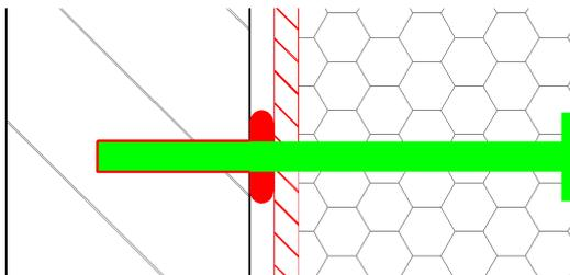
**Figure 9: adhesive (red) injected in hole and gap between wall and insulation**
