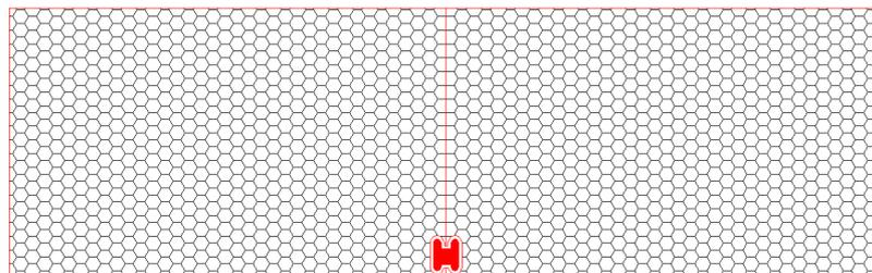
**Figure 8: exemplary block-to-block connection with sealing strip (red) in undercut grooves**
