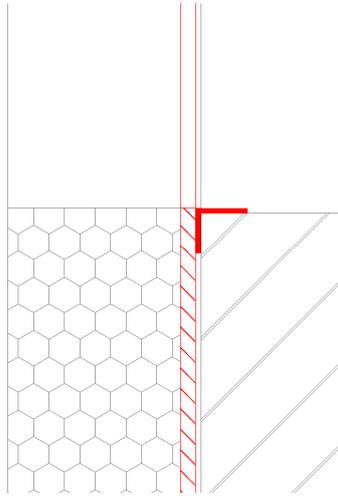
**Figure 13: exterior edge at opening, reinforcing for critical air tightness layer joint (red angle) for window installation at a later date**
