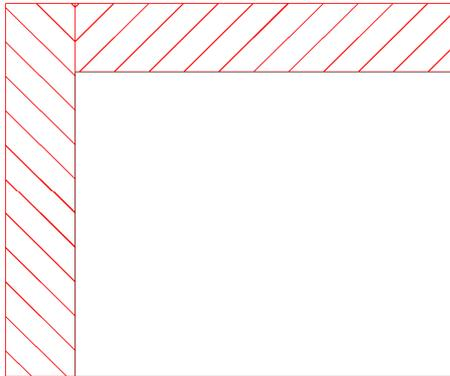
**Figure 6: added sealing/reinforcing tapes (hatched) along two sides of insulation block**
