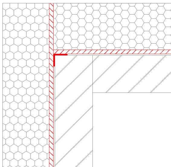
Figure 12: exterior corner, reinforcing joint for critical air tightness layer (red angle)
