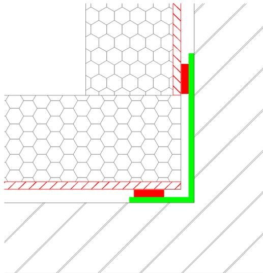
Figure 16: 2.5-2 interior corner with pre-coating/reinforcement/tape (green)
