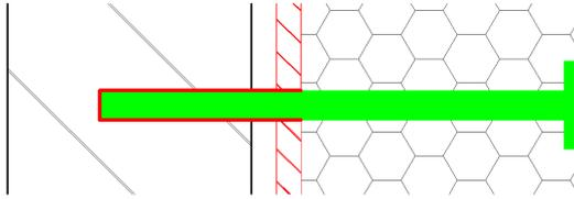
Figure 11: air tight dowel dives into wall and seals with air tight layer of insulation
