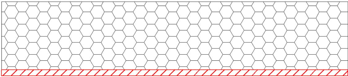
**Figure 3: coated inner surface of insulation block for air tightness**
