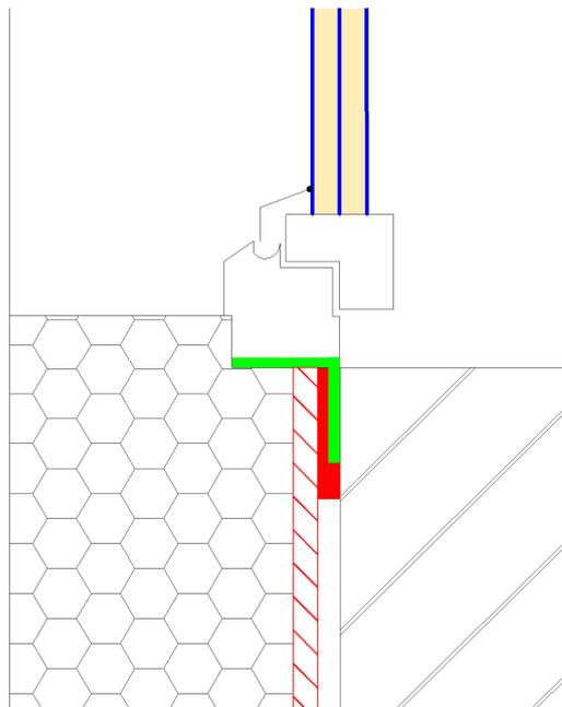
**Figure 14: variation with pre-installed window, window sealing tape (green) accepts insulation adhesive**
