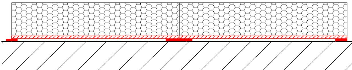
**Figure 5: adhesive (solid red) along respective block perimeter connects air tight layers**
