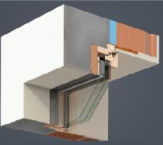
2. When the insulation layer is added, the window is moved to the ideal installation situation.
