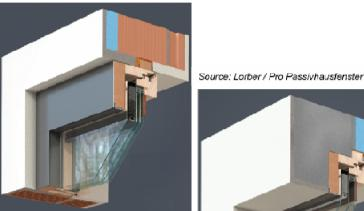
1. New window is installed in the same position as the old window.
