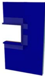
The wood buck needs to be sealed at the corners and connected with self adhesive membrane to the air/water control membrane
