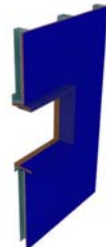
A pre-wrapped treated timber or ply wood buck is added to all four sides of the reveals
