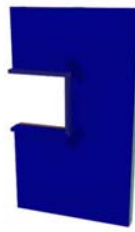
The wood buck needs to be sealed at the corners and connected with self adhesive membrane to the air/water control membrane
