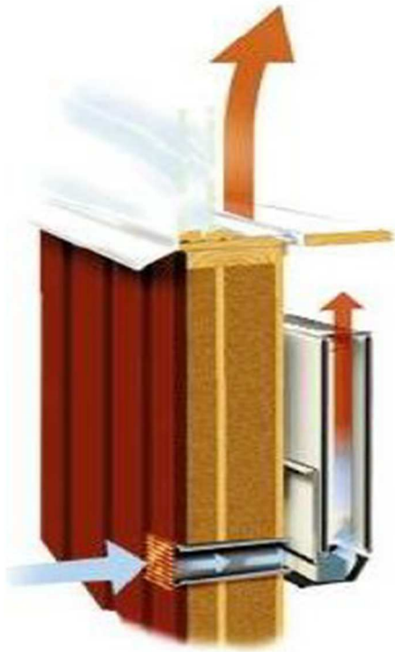
Schematic diagram of a ventilation radiator (Source: Myhren 2011)
