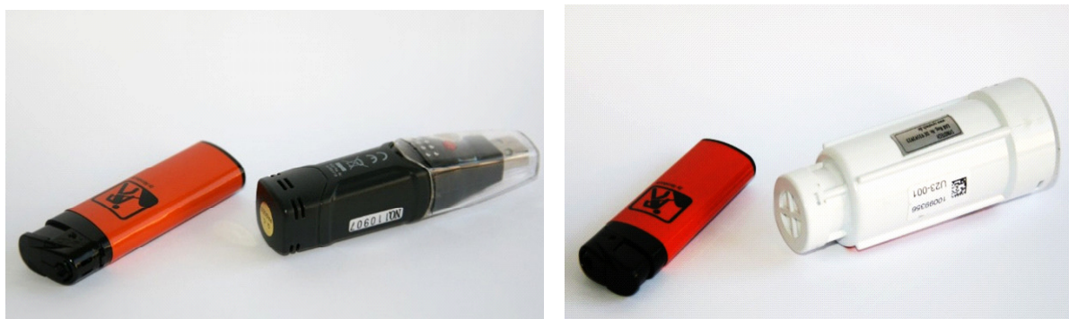
Figure 24: Two examples of different stand-alone data loggers (an ordinary lighter is shown for size comparison)
