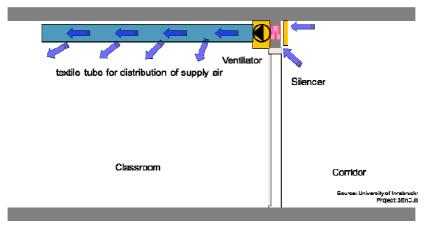
Figure 1: Principle of active air transfer for non-residential buildings from corridor to class [Source: University of Innsbruck/ 3EnCult]
