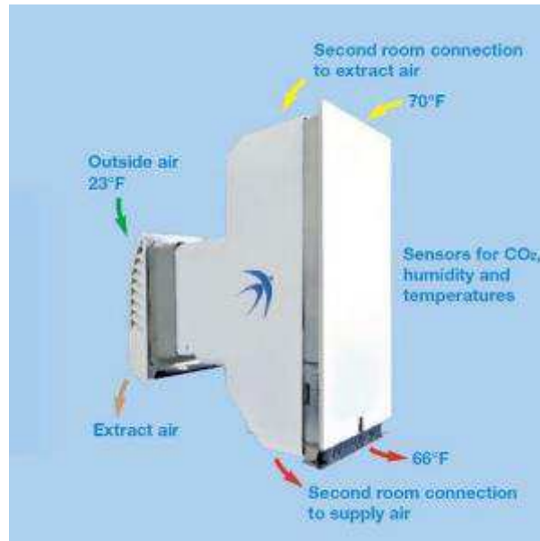
Figure 7: Facade integrated ventilation device with optional second-room-connection [Source: bluMartin]
