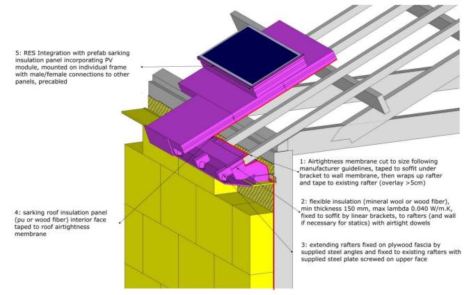
For airtight connection of roof membrane to existing rafters, mastic may be necessary to get the necessary level of adherence.
