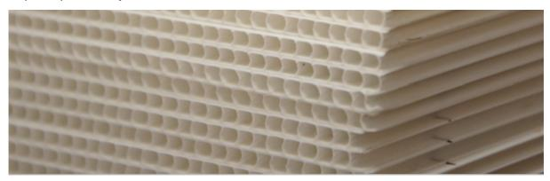
Figure 1: Polypropylene (PP) twin wall panels
