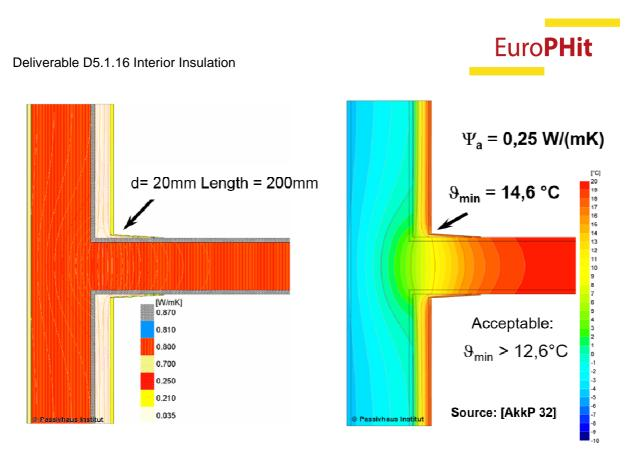
In this case, a "wedge" in the intersection between the wall and the slab allows for a higher surface temperature, reducing the risk of mold formation and/or structural damage.
