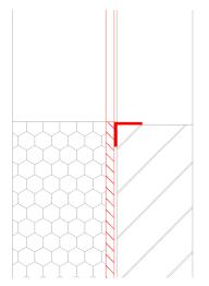
Figure 13: exterior edge at opening, reinforcing for critical air tightness layer joint (red angle) for window installation at a later date
