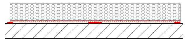
Figure 5: adhesive (solid red) along respective block perimeter connects air tight layers
