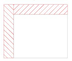
Figure 6: added sealing/reinforcing tapes (hatched) along two sides of insulation block
