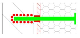
Figure 10: specialised self-sealing dowel
