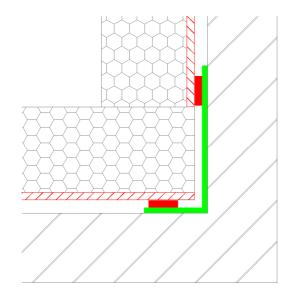
Figure 16: 2.5-2 interior corner with pre-coating/reinforcement/tape (green)
