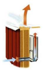
Figure 2: Schematic diagram of a ventilation radiator (Source: Myhren 2011)
