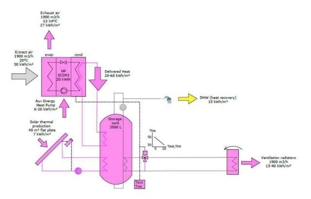
Figure 3: Energy diagram of solution integrating solar thermal panels
